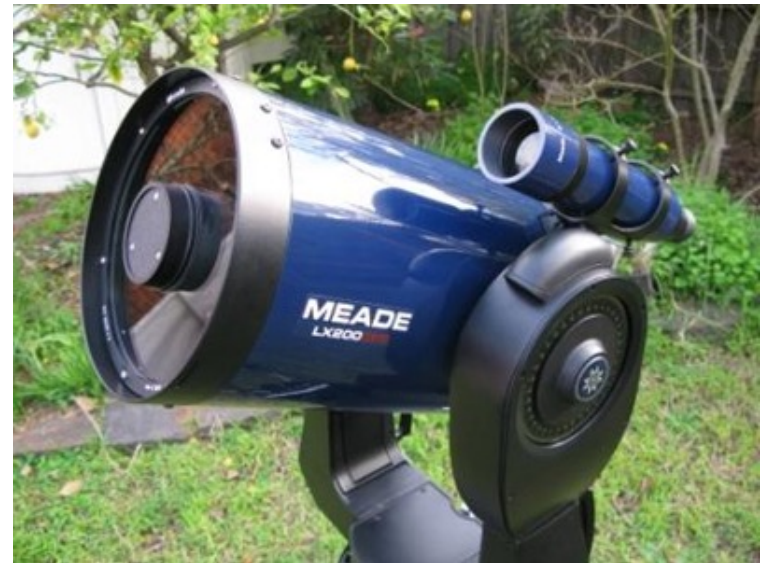
The 8 in reflecting telescope MEADE LX 200.
