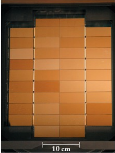
(a) A mosaic of 40 charge-coupled devices (CCDs)
