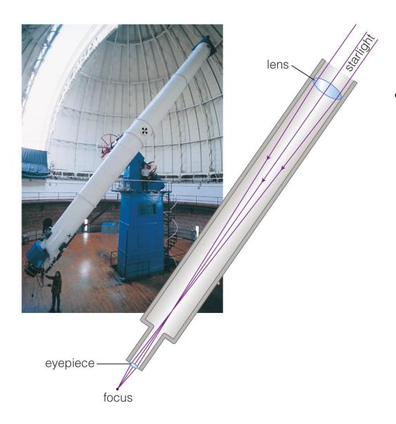
Refracting telescopes need to be very long, with large, heavy lenses.
