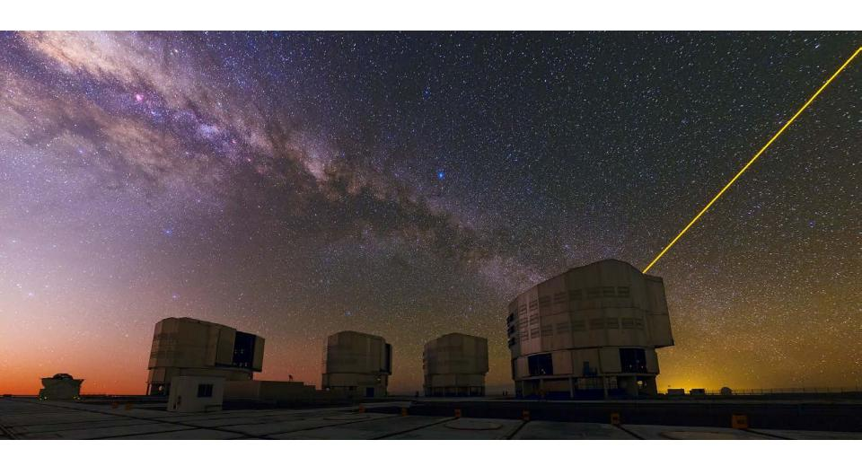
Astronomers can make use of an artificial star by shining a powerful laser to correct for the blurring caused by the atmosphere.
