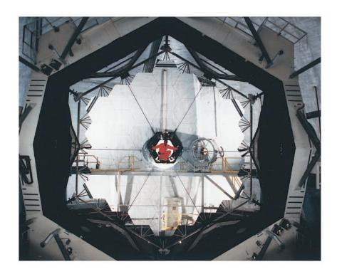
Segmented 10-meter mirror of a Keck telescope
