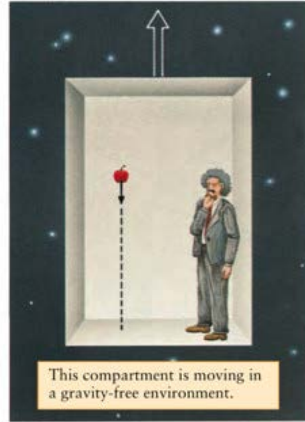
(b) The apple hits the floor of the compartment because the compartment accelerates upward.
